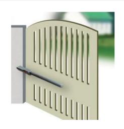
The GM 17 swing gate operator series are used to drive swing gates for industrial, commercial and residential uses. The biggest push power of the device is 1500N, To protect the device, an electric lock is provided to install when the width of gate leaf is more than 1.5 meters. In case of power failure, an emergency release key allows operate gate manually.
